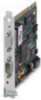
IBS PC ISA SC/I-T PC controller board in ISA format
