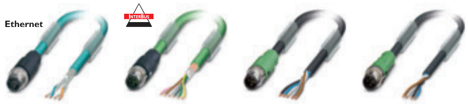
Ethernet Ethernet bus cable 4-pos., D-coded INTERBUS Bus cable local bus FLM M12 5-pos., B-coded, M12-SPEEDCON FLM power cable 5 x 0.75 mm 2 , A-coded, M12-SPEEDCON FLS power cable 4 x 0.75 mm 2 , A-coded, M12-SPEEDCON
