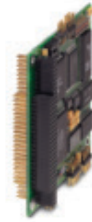
IBS PC 104 SC-T Controller board in PC/104 format
